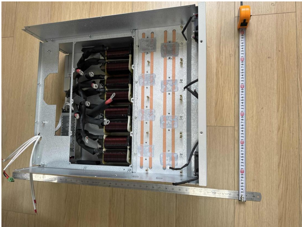
Figure 12 Inside view of enclosure without PCBs
