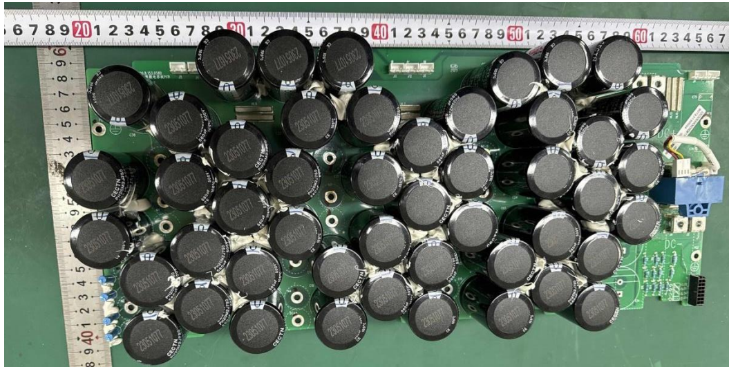
Figure 21 component side of capacitor board
