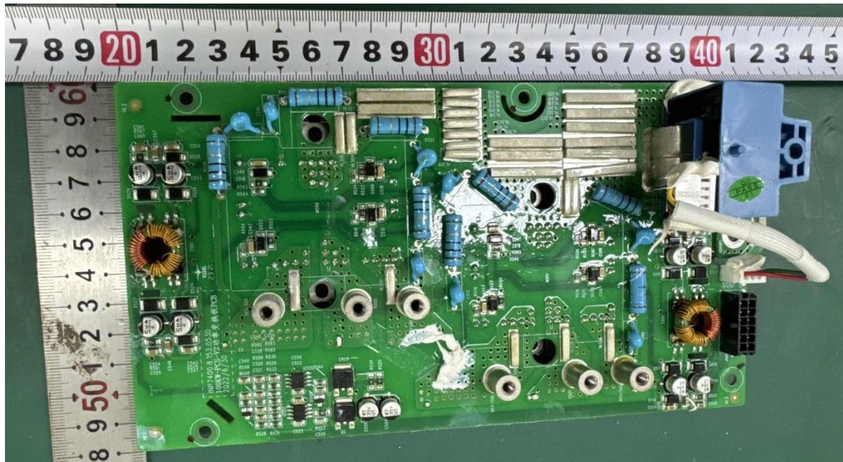
Figure 23 component side of power board
