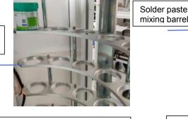
Warming storage rack There are a total of 66 temperature recovery and thawing positions in the 11 layers of the solder paste thawing area, one of which is the place where the solder paste weight block is placed.
