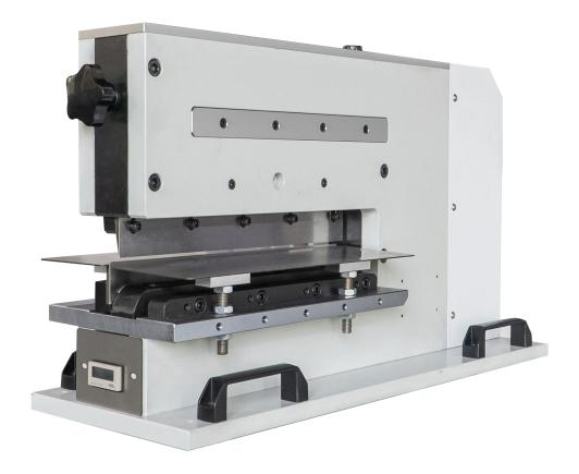
Application Range: Separate precise SMD thin board, aluminum PCB, for special board, please check with Service.
