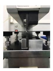
Blade edge of 18 degree, shear of Guillotine type, keep internal stress within 80-180Ue, to avoid micro crack and damage to precise component.
