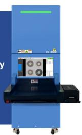
XC-3100 is mainly used for rapid counting of reel-type materials in the SMT industry. It can count all types of materials such as 7-15-inch Tape Reel/JEDEC Tray/IC moisture-sensitive packages. The material types include all resistance-capacitance materials and IC materials. Use X-ray imaging technology to detect production materials and obtain image information for rapid counting, and connect equipment data information with the customer's MES system.
