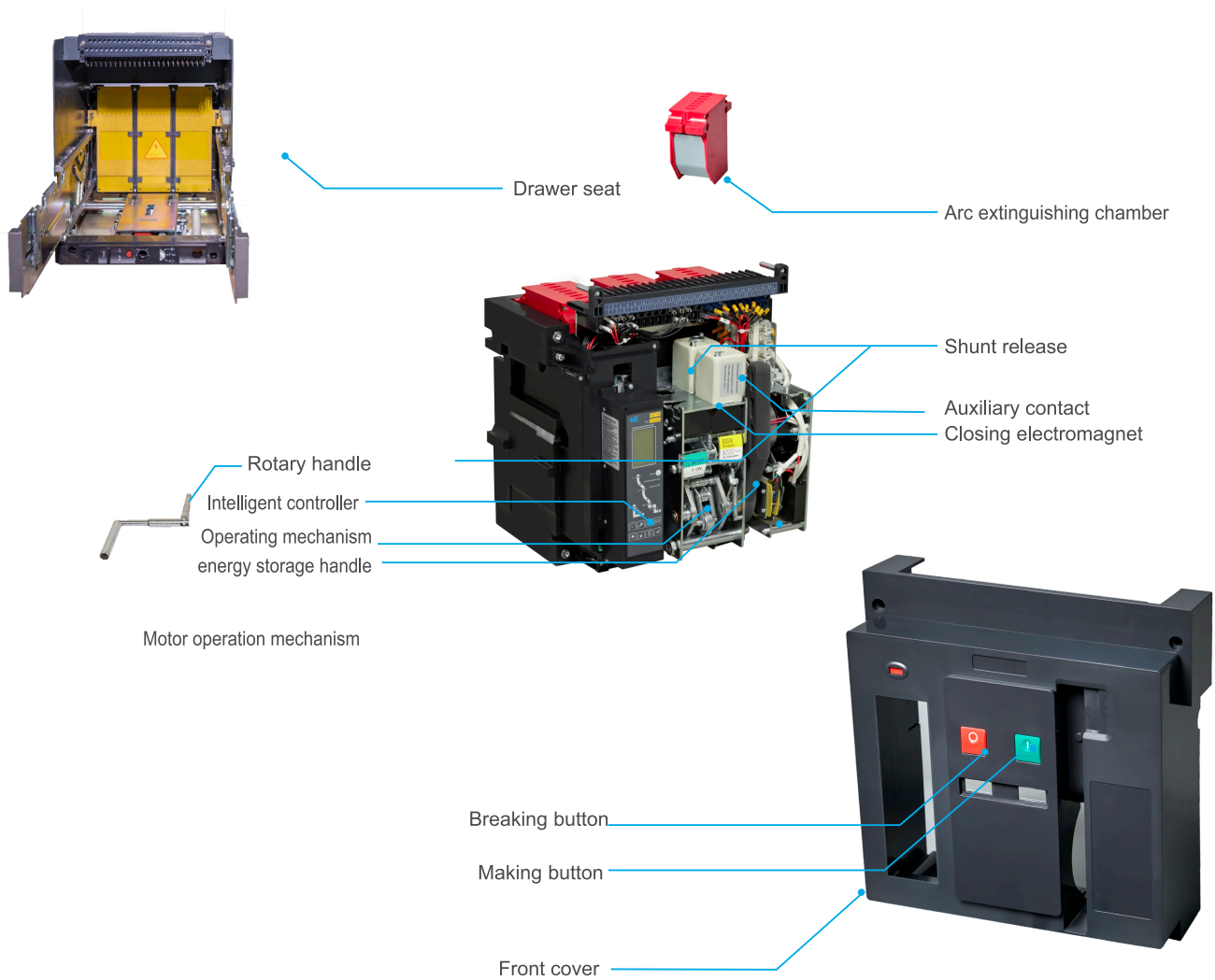
Figure 5.1 WEW1-1600 withdrawable circuit breaker structure
