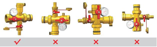
The automatic air vent valves must be installed in a vertical position, with the cap facing upwards. Installation in places that are easy to inspect is recommended.
