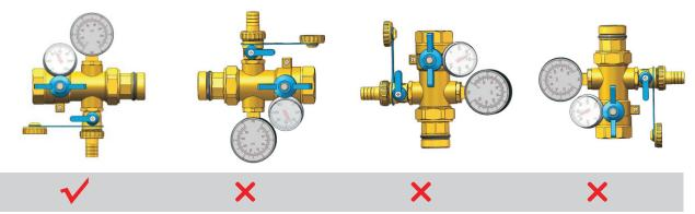
The ZL-4460 series valves are supplied with fluid supply from the left", and can be easily mounted with fluid supply from the right".
