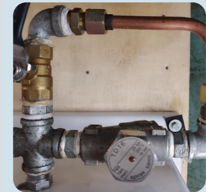
The pressing machine is equipped with a famous brand drain valve with bypass as standard
