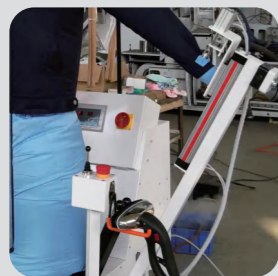
Automatic sleeve stretching mechanism and hanging iron
