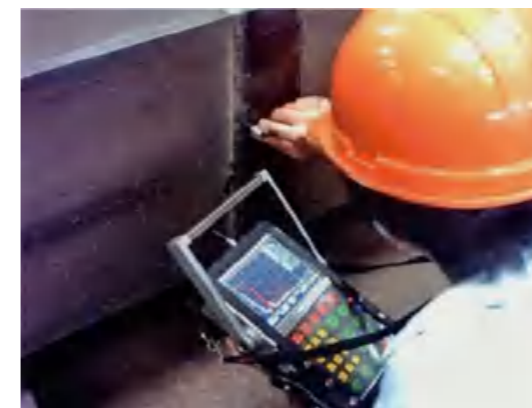
吊臂无损探伤 Boom inspection
