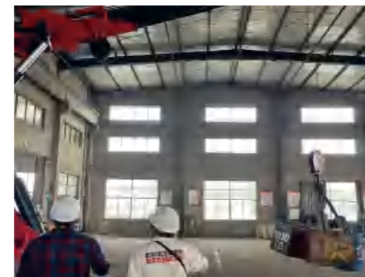
验船师台架检验吊机 Surveyor Bench Test for Crane
