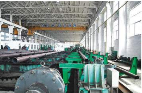
Slight-tensioned reducing mill
