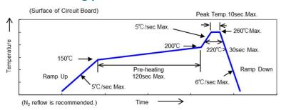
This soldering profile is according to JEDEC-J-STD-020D.
