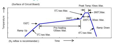
This soldering profile is according to JEDEC-J-STD-020D.
