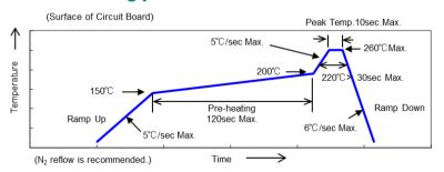
This soldering profile is according to JEDEC-J-STD-020D.
