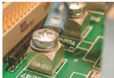
Press-Fit element for currents of up to 160 A
