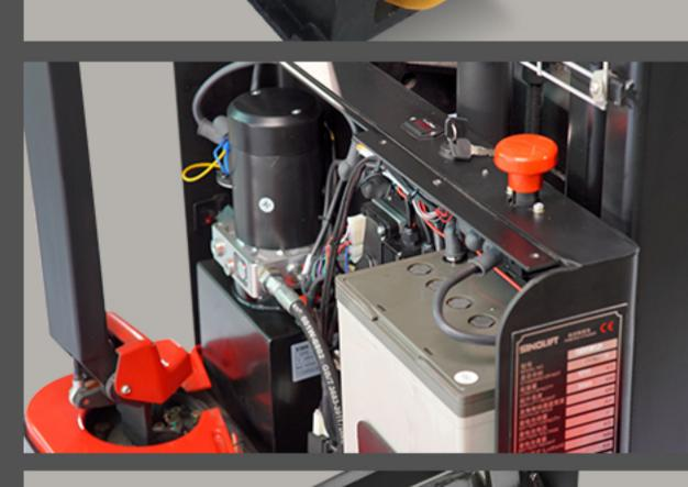
Low-noise and durable hydraulic unit,high quality cylinder as well as hose ensure high reliability of hydraulic system.
