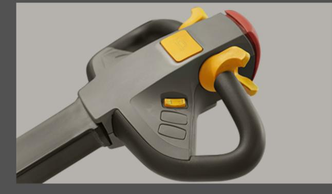
Long tiller arm design helps facilitate a short turning radius and effectively reduces the human effort needed to maneuver the stacker easily.
