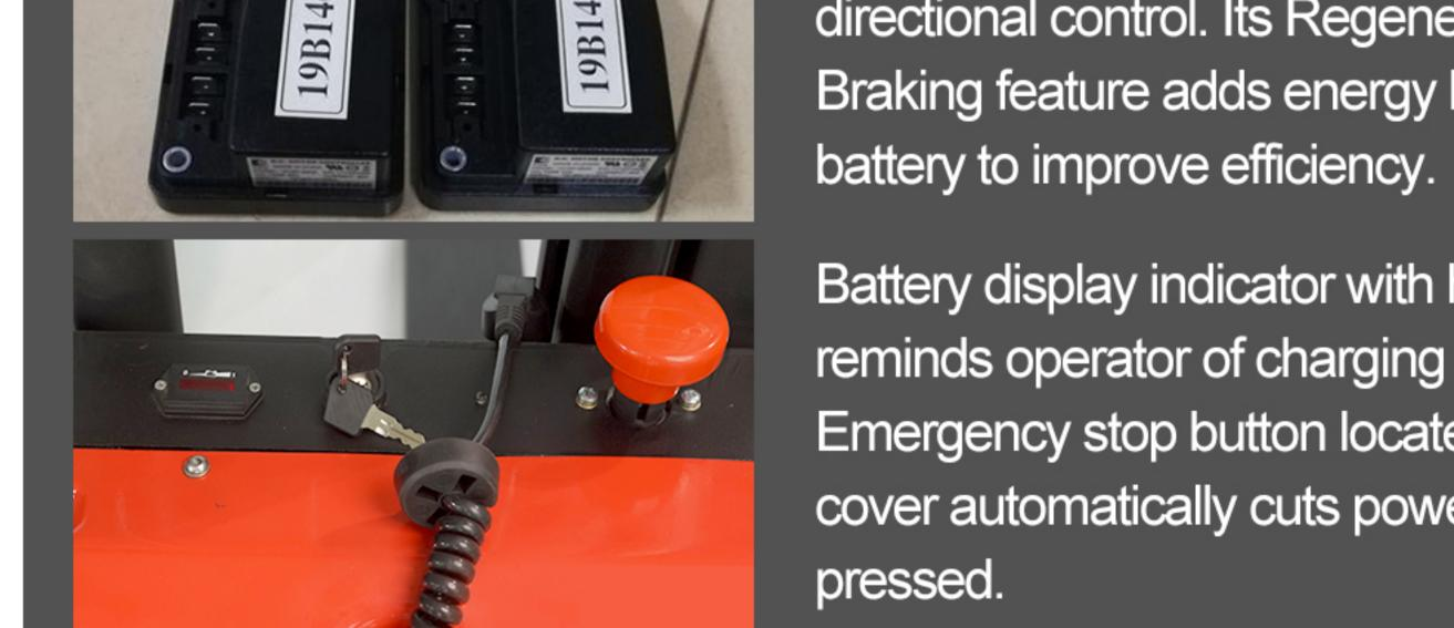
Battery display indicator with hour meter, reminds operator of charging on time. Emergency stop button located on the cover automatically cuts power when pressed.
