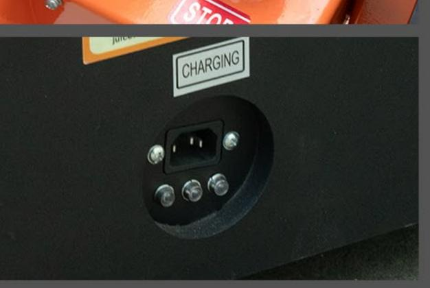
The unit is simple to charge requiring only a standard extension cord to charge.
