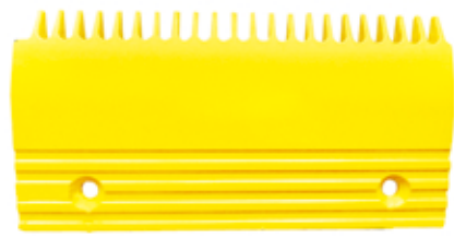
1099# 西子OTIS 22齿ABS梳齿板(左) L47312024A 204×107×孔距145 Xizi Otis 22-teeth ABS Comb Plate (Left)
