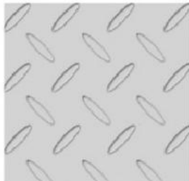
Ordinary checkerd steel plate I (Standard)
