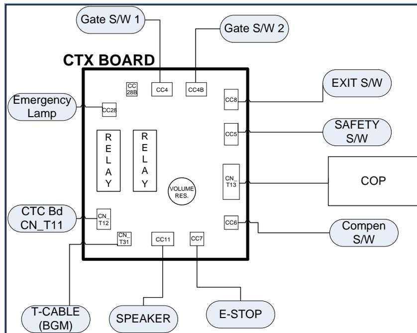
[Figure 5.1 Connection Diagram near CAR Junction Box]
