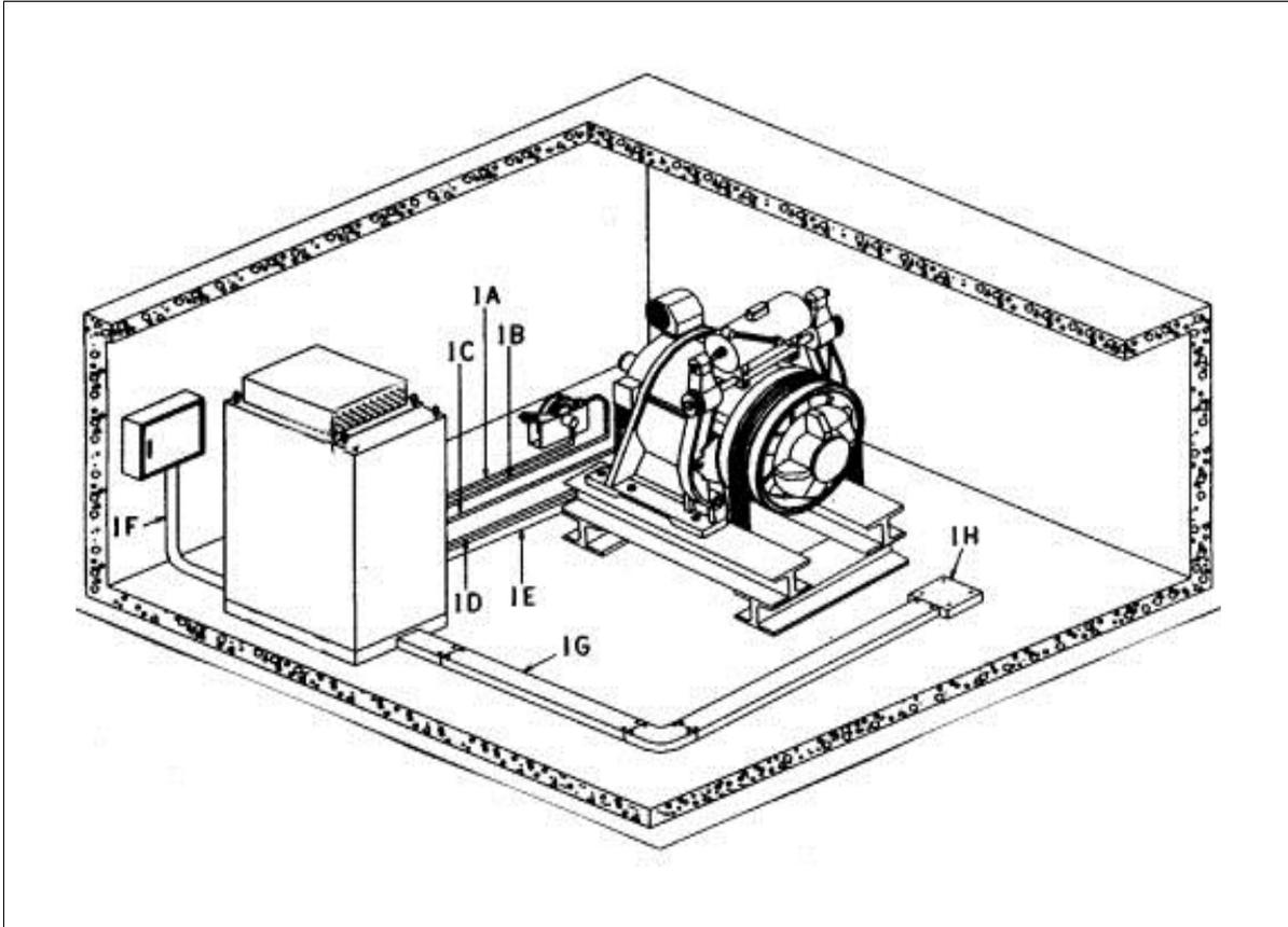
[Figure 3.1 Machine Room Connections and Pipes (Independent Machine Room)]
