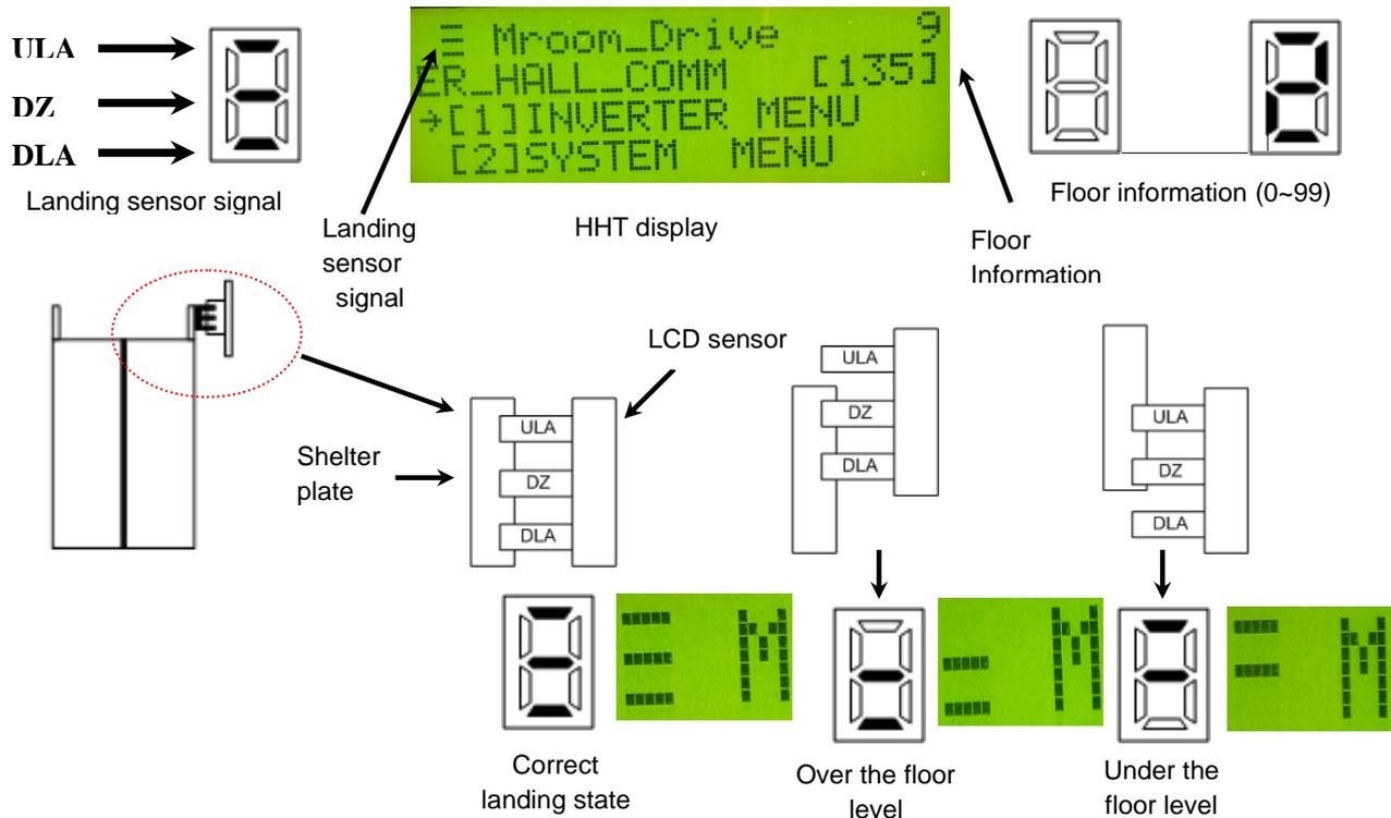
[Figure 7.1 Landing Sensor Information Display]
