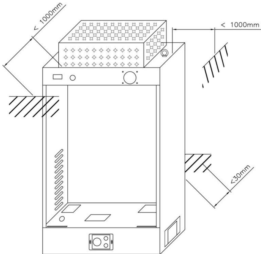
[Figure 2.1 Exterior of CP in Machine Room]
