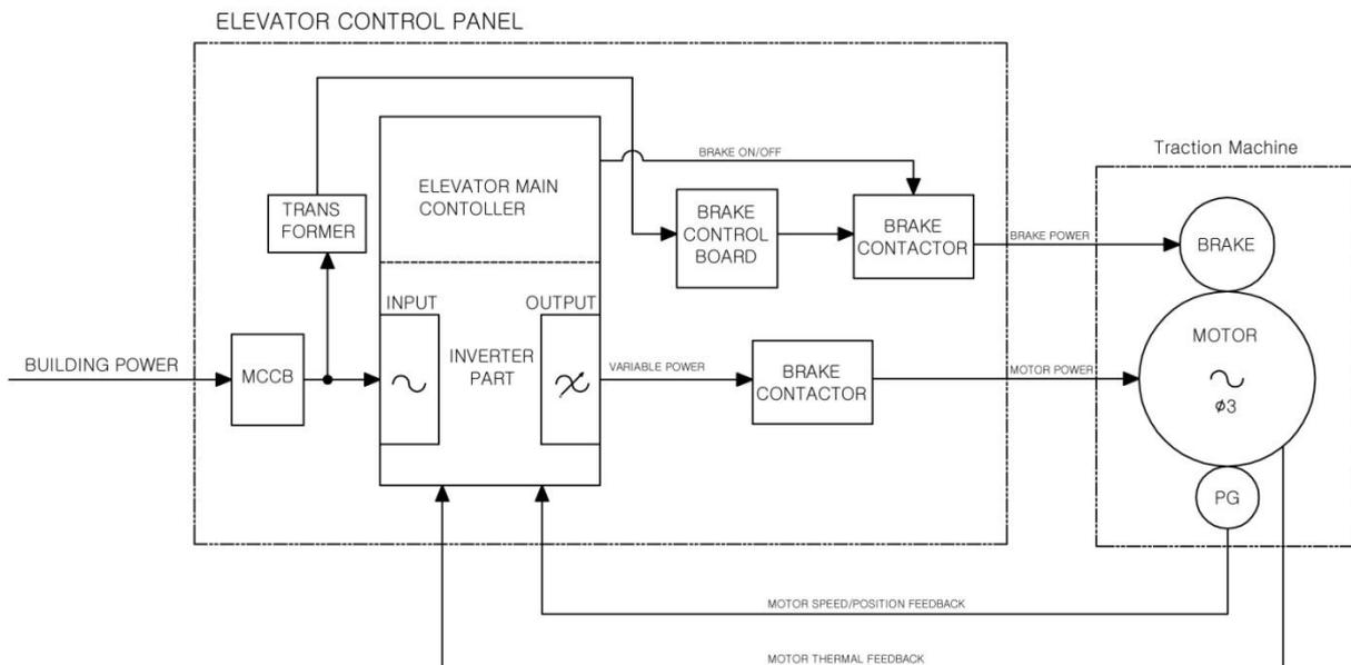
[Figure 1.1 Motor Control Block Diagram]
