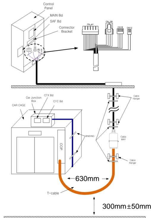
**[Figure 4.1 Traveling Cable (T-Cable) Connection]**
