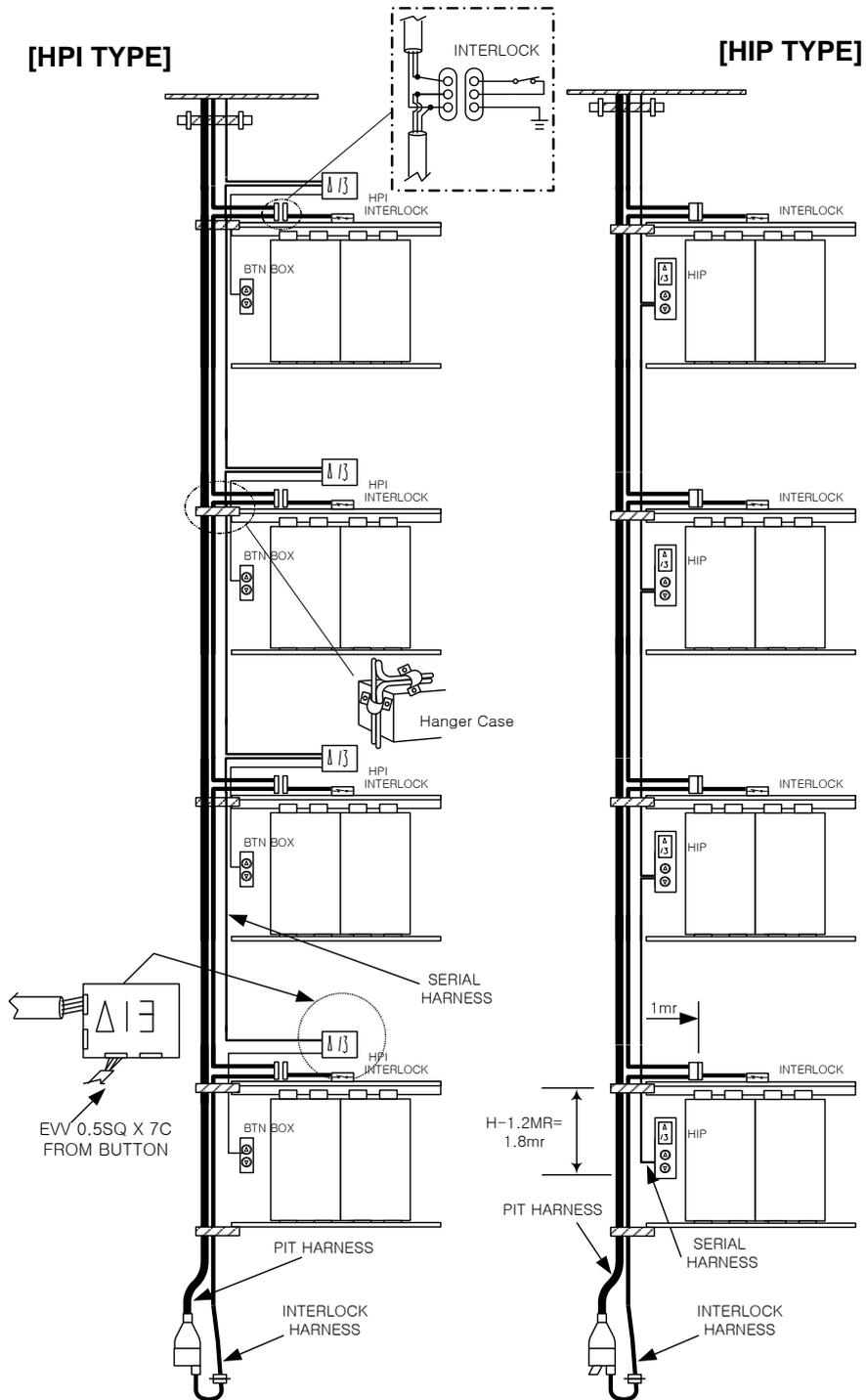
[Figure 4.4 Hoist Way Harness Connection Diagram]
