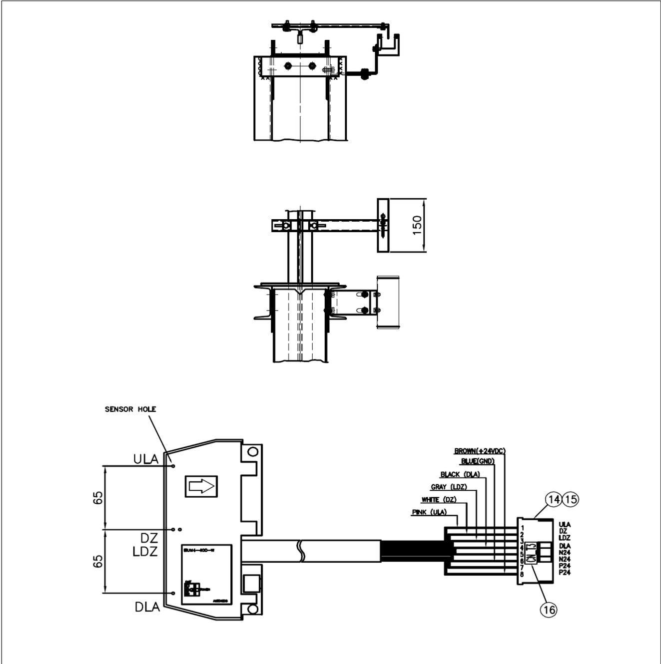
[Figure 5.2 Landing Control Device ASS'Y Mounting Diagram]
