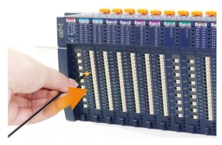
The cable harness is for fixing cables when the I/O module is wired to multiple cables.
