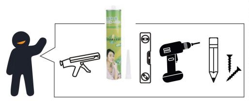
You will need glue and glue chair, spirit level, screwdriver, pencil and black screws. For protection use cotton gloves when working with the panels.
