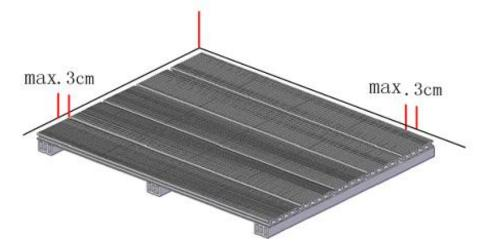
4. The joint kit of decking is stainless steel clips. Drilling should be smaller than the diameter of the screw diameter of 3/4 in order to increase the self-tapping screws grip of the nails.
