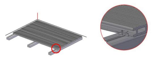
5. Knock the decking gently with the application of rubber hammer during construction to make sure of a equal gap and the beautiful construction surface .
