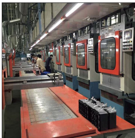
Battery Cast-Welding
