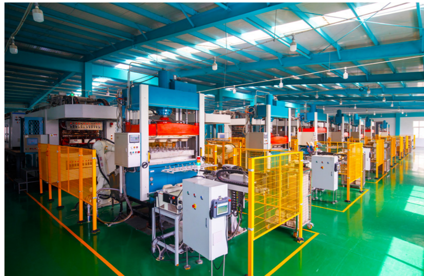
自主研发及制造的全自动数控生产、冲切、覆膜一体机组设备 Fully automated CNC production, punching, and laminating integrated machine units developed and manufactured in-house.
