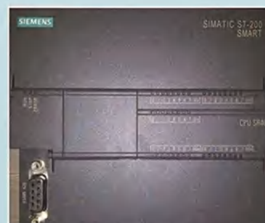
Automatic control PLC mainframe
