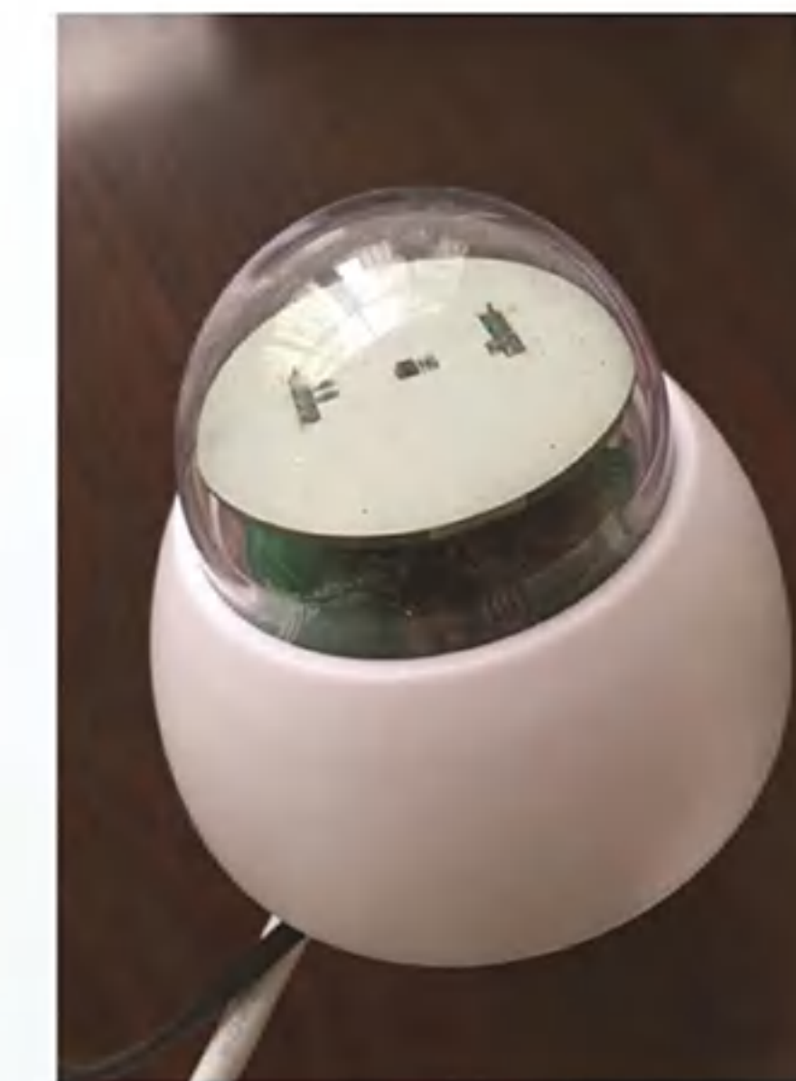
Illuminance, temperature, and humidity sensors
