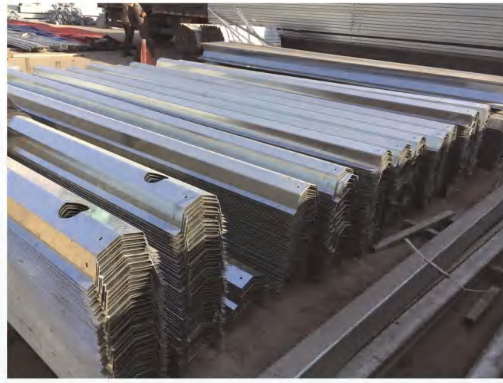
Glass, PC Greenhouse Gutter
