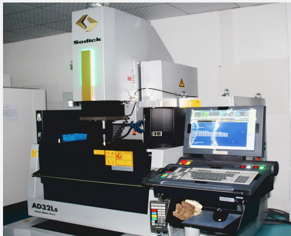
Japan Sodick Spark Machine Precision: 0.005mm
