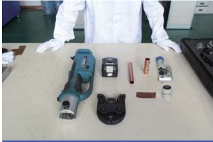
1. Prepare the Pressing tools: Pressing jaw, Pipe cutter, 3M Scouring pad, tube expander, Deburrer
