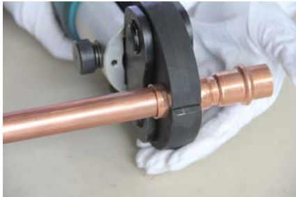
3.Switch to Press when the jaw and fittings is in the right position
