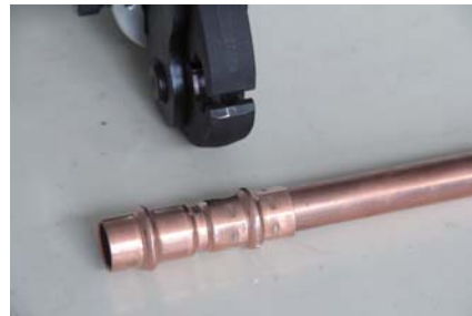
4.The Pressing jaw will be released automatically after finished
