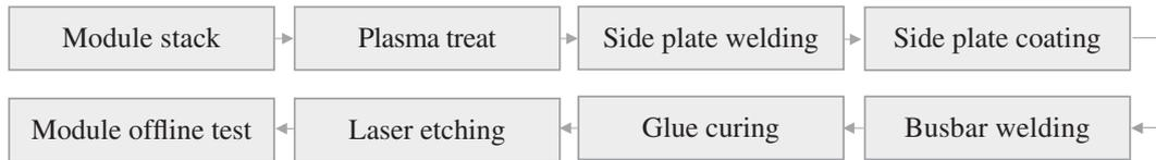
We configured a total of 82 error-proof items for module production and we apply the following technologies in our battery module production process:
