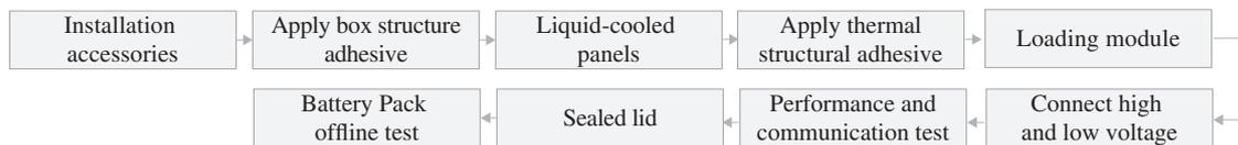
We apply the following technologies in our battery pack production process:
