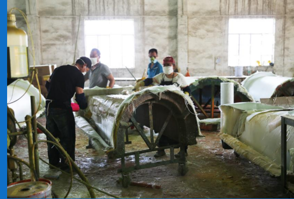
3-Laying fiber on mould
