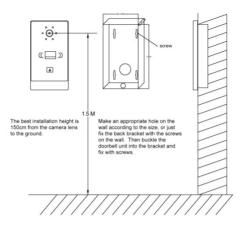
Figure1. Villa Outdoor Doorbell installation schematic diagram
