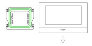
1. Fix the hanging board on the wall or 86 box with screws. The best installation height is 145~160cm from the ground.
