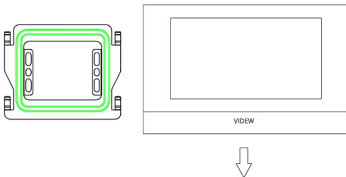
1. Fix the hanging board on the wall or 86 box with screws. The best installation height is 145~160cm from the ground.
