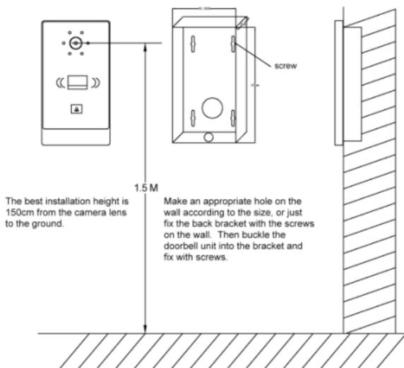
**Figure1. Villa Outdoor Doorbell installation schematic**
