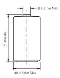
Size unit:mm (GB1804-m if tolerance is not specified)
