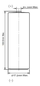
Size unit:mm (GB1804-m if tolerance is not specified)
