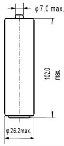
Size unit:mm (GB1804-m if tolerance is not specified)
