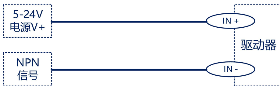
NPN signal connection method
