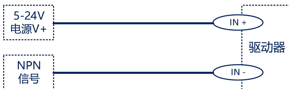
NPN signal connection method
