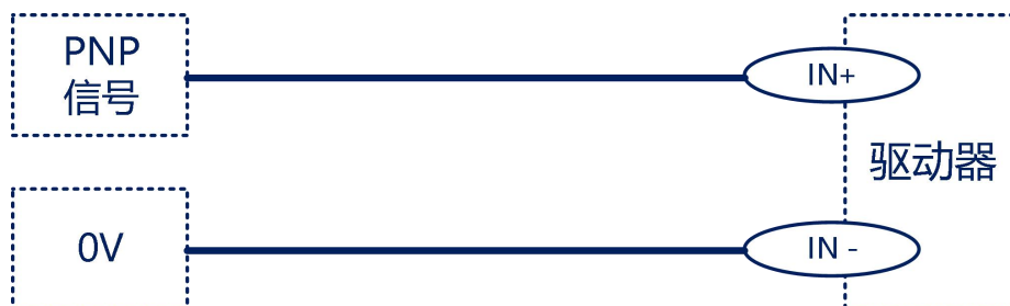
PNP signal connection method
