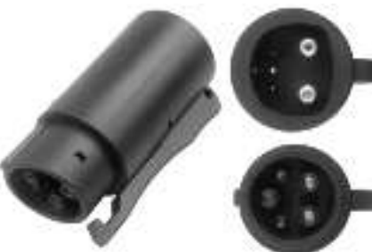
ST-E008 Tesla To Type 1 Adapter Rated Current: 80A Rated Voltage: 110-240V 50~60HZ Application: Used for American standard interface cars in European standard countries
