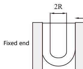
At 20°C, the tube is bent into a U shape, one end is fixed, and the other end is slowly brought closer. The 2R is measured when the tube bends and flattens.
