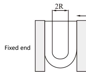
At 20°C, the tube is bent into a U shape, one end is fixed, and the other end is slowly brought closer. The 2R is measured when the tube bends and flattens.
