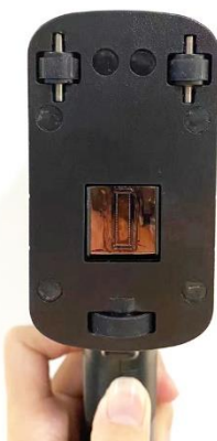
3. Put it into the ink tank at a 45° angle and press it down
