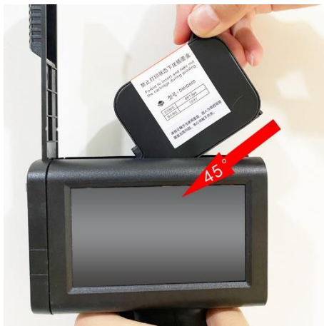
3. Put it into the ink tank at a 45° angle and press it down
