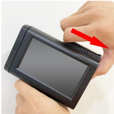
1. Open the ink tank cover and push it back in parallel to open
