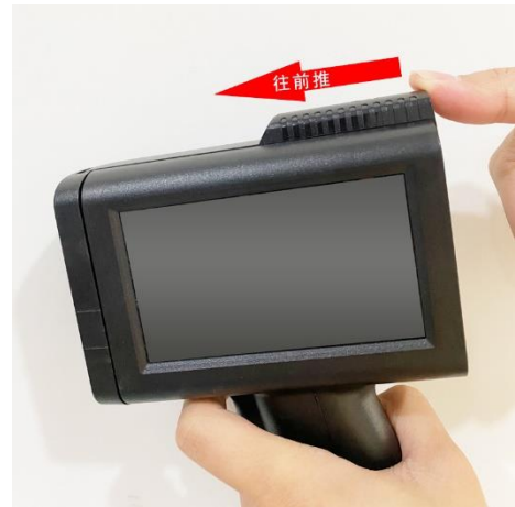
2. Open the transparent protective cover of the ink cartridge
