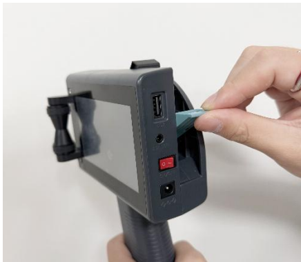
3. Then snap the lever on and tighten the cartridge
