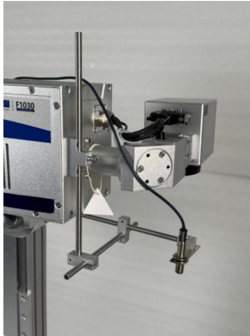
The Photoelectric Sensor And Its Bracket Have Been Installed
