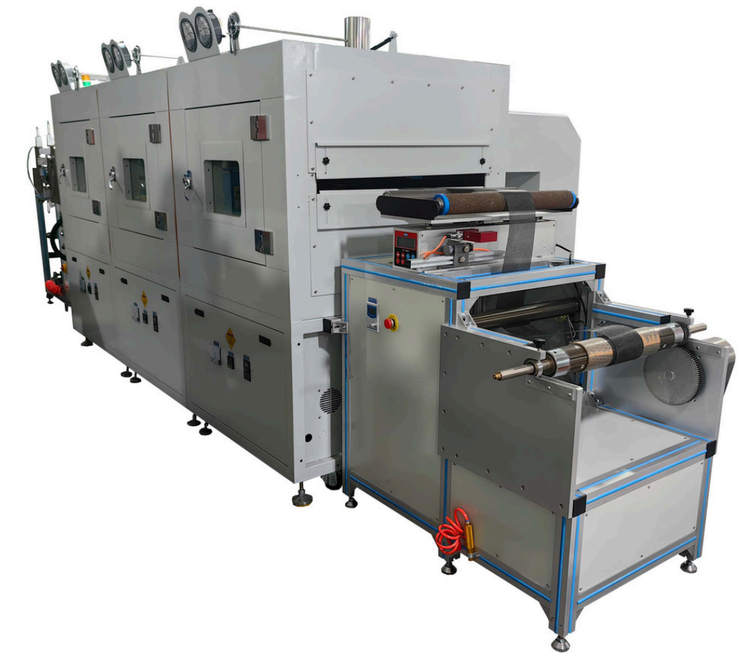
Custom Double-Sided Coating Machine with Suspension Oven
