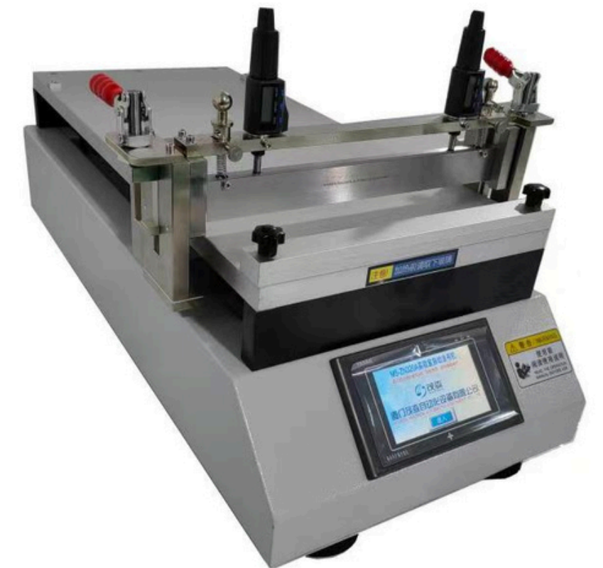
Experimental Doctor Blade Automatic Small Testing Coating Machine
