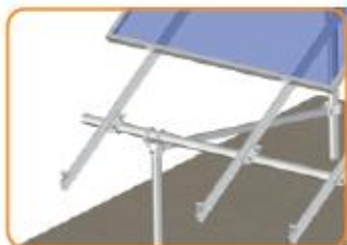
Rail & pipe connection
