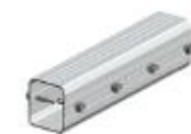
AS-TRS-35B TR-35B rail splice W45.5*H52.8mm Material: aluminum 6005-T5 Self drilling bolt M6.3*25mm 8pcs Application: AS-TR-35B
