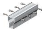
AS-RS-16 Rail 16# & Rail 17# splice L=220mm Material: aluminum 6005-T5 Self drilling bolt M6.3*25mm 8pcs Application: AS-R-16/17
