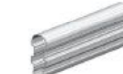
AS-WHC-01 Rail jointer W1# L=300mm Material: aluminum 6005-T5 Self drilling bolt M6.3*25mm 8pcs
