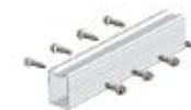
AS-TRS-65 TR65 rail splice L=200mm Material: aluminum 6005-T5 Self drilling bolt M6.3*25mm 8pcs Application: AS-TR65
