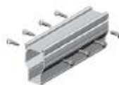
AS-RS-14 Rail 14# splice L=220mm Material: aluminum 6005-T5 Self drilling bolt M6.3*25mm 8pcs Application: AS-R-14
