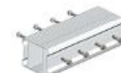
AS-ABS-D10 Aluminum beam 10#splice L=220mm Material: aluminum 6005-T5 Self drilling bolt M6.3*25mm 8pcs Application: AS-AB-D10
