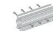
AS-TRS-105 TR105 rail splice L=220mm Material: aluminum 6005-T5 Self drilling bolt M6.3*25mm 8pcs Application: AS-TR105
