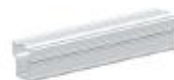
AS-WHC-03 W Rail 3# Rail jointer L=200mm Material: aluminum 6005-T5 Self drilling bolt M6.3*25mm 4pcs Application: AS-W-H03, AS-W-H03-T
