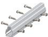
AS-RS-13 Rail 13# splice L=300mm Material: aluminum 6005-T5 Self drilling bolt M6.3*25mm 8pcs Application: AS-R-13
