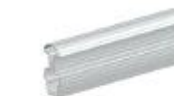
AS-WHC-04 W Rail 3# Rail jointer L=200mm Material: aluminum 6005-T5 Self drilling bolt M6.3*25mm 4pcs Application: AS-W-H04, AS-W-H04B
