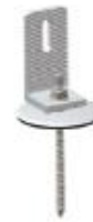
AS-RH-02RP Asphalt shingle roof hook Width of L feet: 40mm Dimension of round plate: \phi 76 Hanger bolt M8x135 Application: asphalt shingle tile roof
