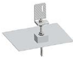
AS-RH-02P Asphalt Tile Roof Flashing L Feet Width of L feet: 50mm Size of aluminum plate: 250*200mm Size of aluminum pad: 50*40*33mm Hanger bolt M10*200 / M10*300 Application: asphalt shingle tile roof
