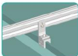
Panel fixed on the rail, rail is perpendicular to the roof rib.
