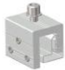
AS-N4-50 N Clip 4# L50*W38*H42mm Material: aluminum 6005-T5 Application: metal / tin roof
