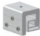
AS-N5B-50 N Clip 5B# L50*W38*H42mm Material: aluminum 6005-T5 Application: metal / tin roof
