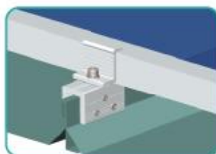
Panel fixed on the roof clip without rail.
