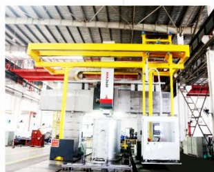
◆ 12米数控动梁龙门镗铣床 12m Cnc Gantry Boring & Milling Machine With A Movable Cross Rail
