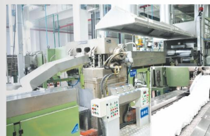
⑤ H2/HD3184型大容量卷曲机 H2/HD3184 High capacity Crimper
