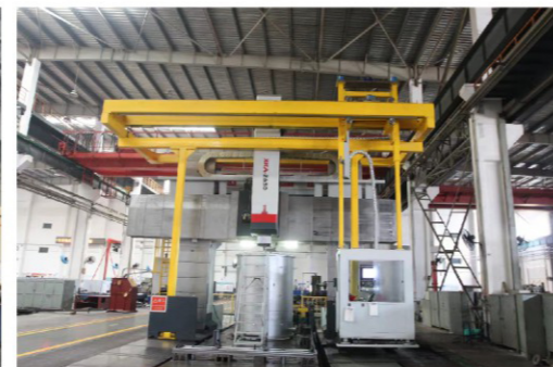
12米数控动梁龙门床 12m CNC Gantry Boring&Milling Machine with amovable crossrail
